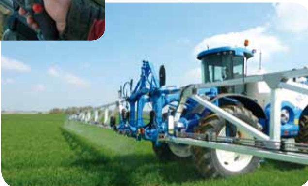
Section cut-off done manually through the console or the forward handgrip (optional) or automatically through DGPS (optional).
